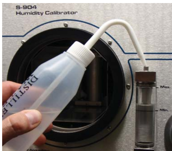
Figure 9 Filling the Water Reservoir
